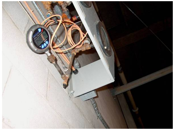
Calibration of transducer and gauge.
