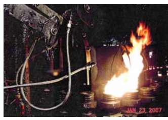
Molten glass poured into a mold at a glassware manufacturer.
