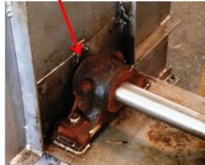
Leakage through seal causing bearing damage
