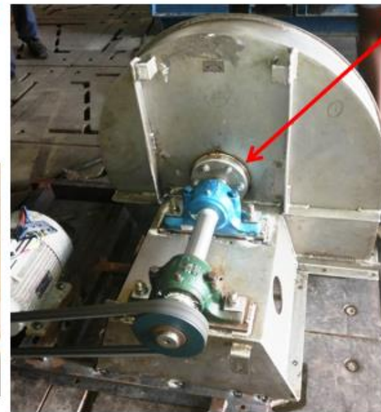
Leakage through seal causing bearing damage
